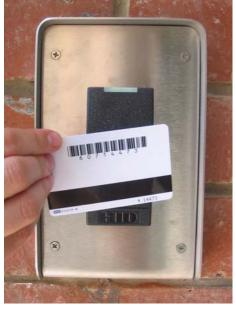
If your card is accepted, the reader light will go solidly green for a few seconds while the door is unlocked. This is shown in the picture below.
